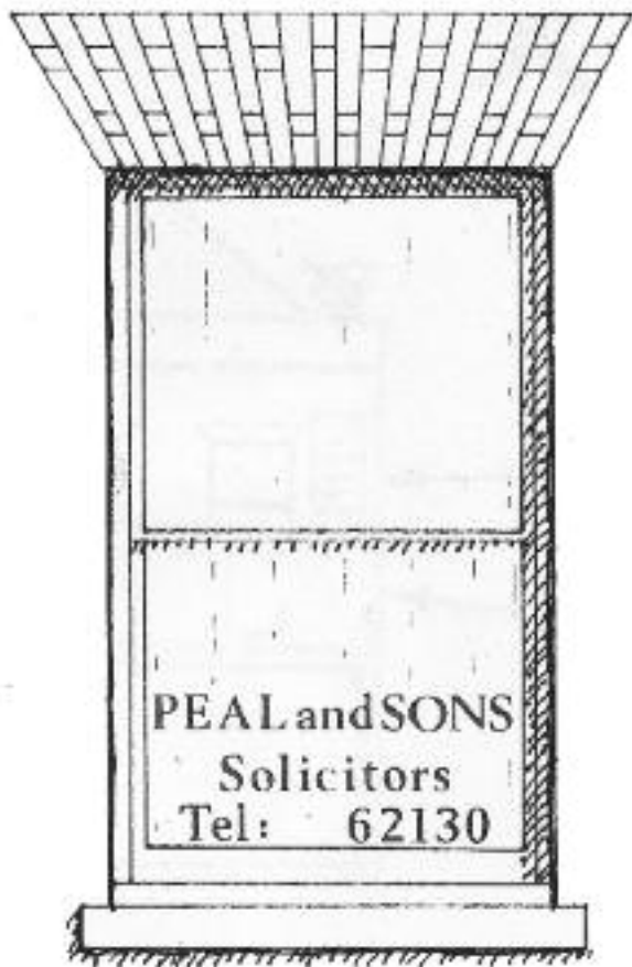
FIG.24. Example of lettering applied to window pane.
